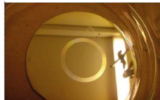
Reflective ring of 64 CGH frames on Silicon wafer
