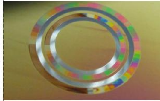
Special purpose photo mask — combination of amplitude and phase type
